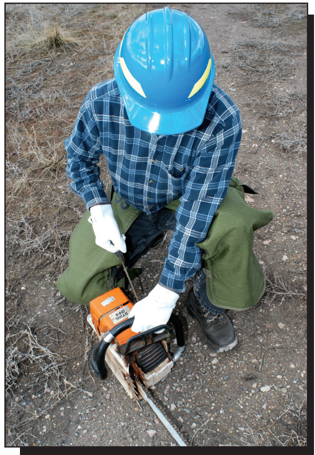
Figure 3-17—Start the saw on firm ground.
