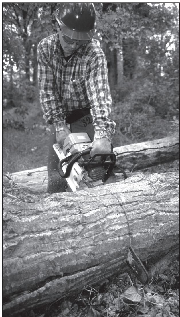
Figure 4-11—Watch the kerf for movement that will indicate a bottom bind (kerf opens) or top bind (kerf closes).
