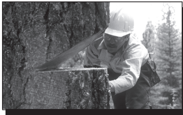
Figure 4-23—The sloping cut is a 45-degree angle.
