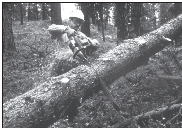
Figure 4-2—The top side of suspended logs should be limbed while you are standing on the ground or you can buck the log to lower it to the ground before limbing.
