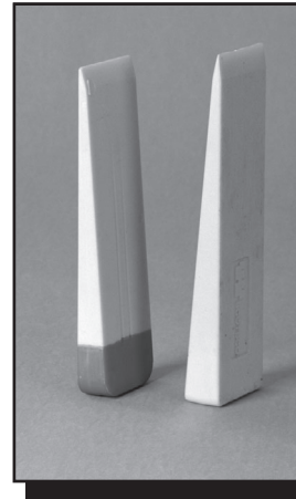
Figure 5-13—Double-taper wedges are designed to reduce bind.
