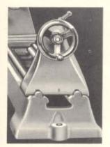
The massive bed and finely machined ways give accurate and positive alignment. Sturdy tallstock has large hand wheel and quill lock.
