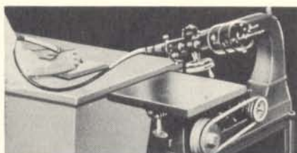
Doing carving with the head in vertical position. Beautiful relief carvings may be produced easily. Pattern guides the work.
