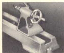
Sturdy tailstock has graduated steel ram.
