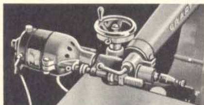
Router head assembly tilted for spindle carving. Scale on head shows angle. Uses cutters below. Does a wide variety of work.
