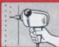
Drill holes up to 3/4-in. diameter in metal; up to 1-in. diameter in wood
